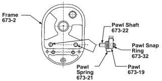
K. Slide friction hub (673-12) onto pinion (673-9) and place one friction disc (673-13) on top of friction hub. Assemble ratchet bushing (673-24) to rachet (673-23). Spring apart pawls and slide ratchet/bushing assembly on friction hub as shown below.
