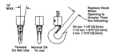
On latch type hooks, check to make sure that the latch is not damaged or bent and that it operates properly with sufficient spring pressure to keep the latch tightly against the tip of the hook and allow the latch to spring back to the tip when released. If the latch does not operate properly, it must be replaced. See above illustrations to determine when the hook must be replaced.
