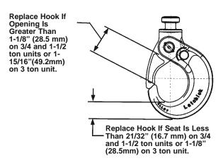
On Latchlok type hooks, measure seat wear and throat opening as shown above and replace hook if measurements indicate the need to do same.
