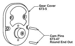
H. Assemble the cam (673-18) to the gear cover (673-5) so that the arrow is pointing towards "operate".
